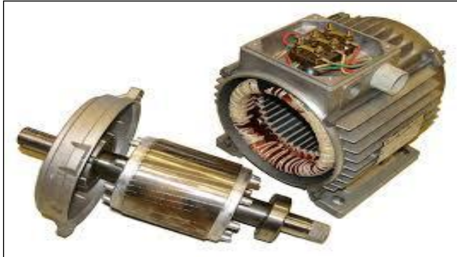
Figure I.2 : Constitution de la machine asynchrone, [6].
